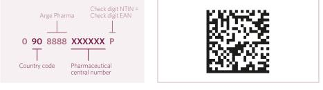
Image 6: NTIN-structure with "leading O" for the GS1 Data Matrix code, based on the EAN-13 code
