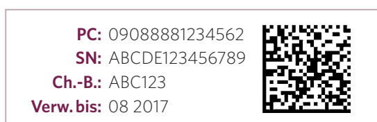
Image 9: Data matrix code with human readable text elements
